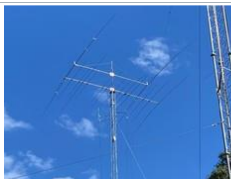
Tower 1 of the Tampa Amateur Radio Club, with the Force 12 C31XR antenna, second from the top. [Lu Romero, W4LT, photo.]
