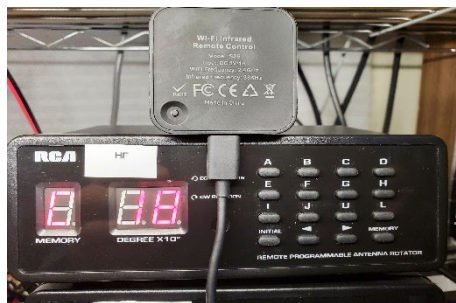
Picture 2 RCA VH226E Rotator Box. Sitting on top is the IR hub, it hangs out in front of the rotator box about 6 inches away, just on top of box for the picture.
