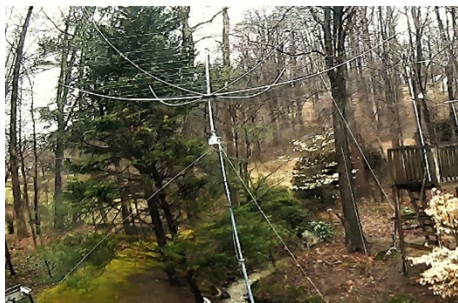
Picture 1 RCA VH226E Antenna Rotator mounted hexbeam antenna.
